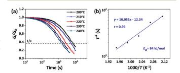
Fig. 3 (a) The normalized stress relaxation of CPA/ESO networks (R = 1.25, TBD 5 mol%) at 200, 210, 220, 230, and 240 °C, respectively. (b) Fitting of the experimental values of relaxation times ( $\tau^*$ ) derived from (a) to an Arrhenius-type equation.
