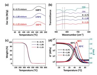
Fig. 2 (a) The DSC curves of the CPA/ESO mixtures at a heating rate of 5 °C min<sup>-1</sup>. (b) The FTIR spectra of the ESO, CPA, and CPA/ESO networks. (c) The TGA curves of the CPA/ESO networks at a heating rate of 10 °C min<sup>-1</sup>. (d) Storage modulus (G', squares) and  $\tan \delta$  (circles) values of the CPA/ESO networks. R = 0.75, 1.00, and 1.25. The concentration of TBD was 5 mol%.
