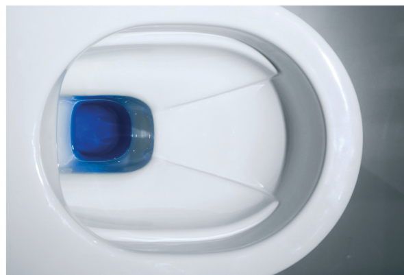
Fig. 3 The urine-separating toilet safe! from LAUFEN, implementing the urine trap. The special structures at the front-end of the toilet direct the urine towards the (nearly invisible) urine trap. 112 Copyright LAUFEN. 123
