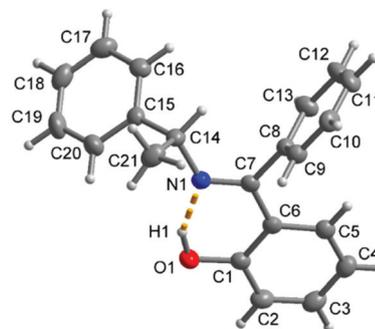
Fig. 3 Molecular structure of  $R\text{-HL}^1$  with the dashed orange line showing the intramolecular hydrogen bond with  $\text{O1-H1}$   $0.91(2)\text{ \AA}$ ,  $\text{H1}\cdots\text{N1}$   $1.70(3)\text{ \AA}$ ,  $\text{O1}\cdots\text{N1}$   $2.533(2)\text{ \AA}$ ,  $\text{O1-H1}\cdots\text{N1}$  angle  $151(2)^\circ$ .
