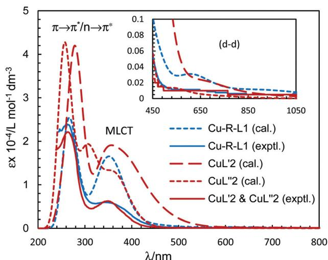
**Fig. 7** Experimental UV-Vis spectrum for Cu-*R*-L<sup>1</sup> (identical to Cu-*S*-L<sup>1</sup>) (0.04 mM) and CuL'<sub>2</sub>/CuL''<sub>2</sub> (0.05 mM) in chloroform at 25 °C. Calculated spectra for  $\Lambda$ - or  $\Delta$ -Cu-*R*-L<sup>1</sup>, CuL'<sub>2</sub> and CuL''<sub>2</sub> at the m06/sdd//b3lyp/6-31 g(d) level with PCM in chloroform (Gaussian band shape with exponential half-width,  $\sigma = 0.33$  eV).
