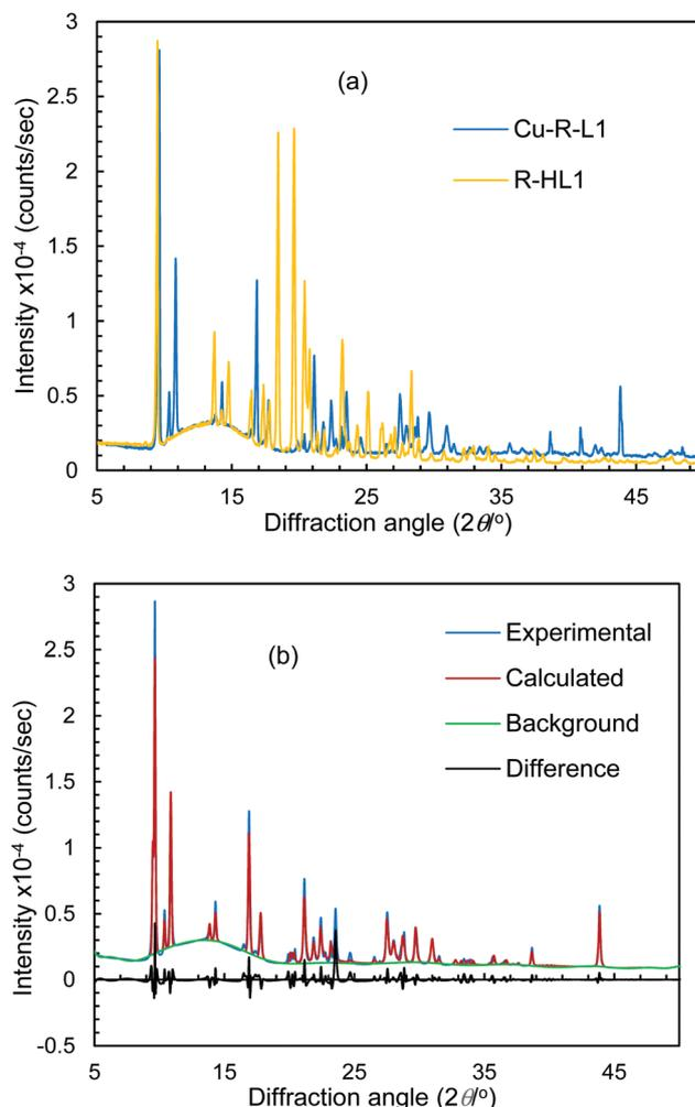
Fig. 5 (a) PXRD patterns for  $R-HL^1$  and  $Cu-R-L^1$ . (b) Experimental and calculated Rietveld refinement plots for  $Cu-R-L^1$  (calculated for  $\Lambda$ - $Cu-R-L^1$ ; see Fig. S8, S9, ESI† for  $R-HL^1$  and  $\Delta$ - $Cu-R-L^1$ ).
