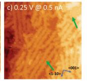
Fig. 3 STM images showing overviews of the Ag(110) surface covered by a sub-monolayer of GNRs and subject to different treatments: (a) pristine GNRs; (b) same as (a) after exposure to  $O_2$  at room temperature; (c) same as (a) after exposure to  $O_2$  at 300 °C. The nominal  $O_2$  dose is always 900 L (~4500 L when considering the doser enhancement factor). The green arrows in (c) point to additional features forming both in-between the GNRs and on bare Ag(110) areas.
