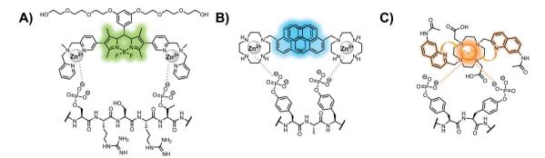
Fig. 7 Main binding mechanisms of sensors for proximal phosphorylation. (A) Two or more Zn(II)-chelate receptors within one sensing scaffold binding to a proximal phosphorylation motif; (B) two individual Zn(III)-chelate receptor molecules detecting proximal phosphosites with excimer reporting; (C) lanthanide binding to phosphosites with antenna sensitization.
