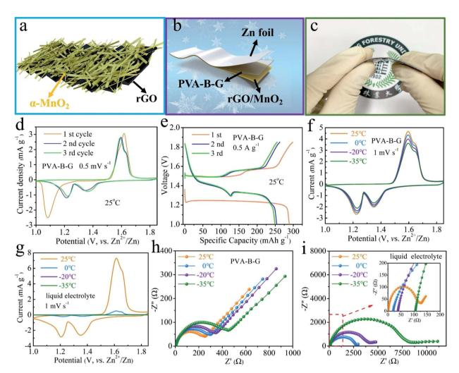
Fig. 3 (a) Graphic illustration of the rGO/MnO<sub>2</sub> nanocomposite. (b) Schematic diagram, (c) photograph, (d) CV curves of the initial three cycles at 0.5 mV s<sup>-1</sup> at 25 °C, and (e) GCD curves of the initial three cycles at 0.5 A g<sup>-1</sup> at 25 °C of the PVA-B-G battery. (f and g) CV curves at 1 mV s<sup>-1</sup> and (h and i) Nyquist plots of (f and h) PVA-B-G battery and (g and i) liquid-electrolyte battery at different temperatures.
