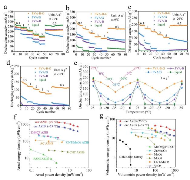
Fig. 4 Rate performances of PVA-B-G, PVA/G, PVA-B, and liquid-electrolyte batteries: (a) at 25 °C, (b) at 0 °C, (c) at -20 °C, and (d) at -35 °C. (e) Cyclic testing results of four types of batteries at 25, 0, -20 °C, and -35 °C at 1 A  $g^{-1}$ . (f) Areal and (g) volumetric Ragone plots of our PVA-B-G battery, in comparison with previously reported energy storage devices.
