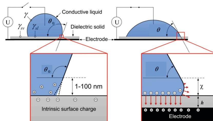
Fig. 2 Schematic of the electrowetting of a conductive liquid droplet on a substrate. Reproduced with permission from ref. 72. Copyright 2012, Taylor & Francis.<sup>72</sup>
