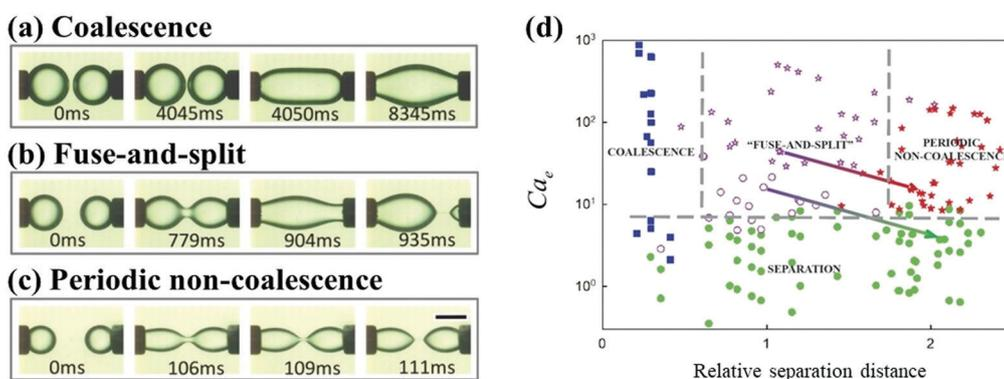
Fig. 7 As the separation distance between two droplets increases, the dynamic regimes of (a) classical coalescence, (b) fuse-and-split, and (c) periodic non-coalescence occur in sequence.<sup>116</sup> (d) State diagram for the dynamic behaviors of droplet pairs, based on the electrocapillary number  $Ca_e$  and the relative separation distance.<sup>116</sup> Reproduced with permission from ref. 116. Copyright 2015, AIP Publishing.
