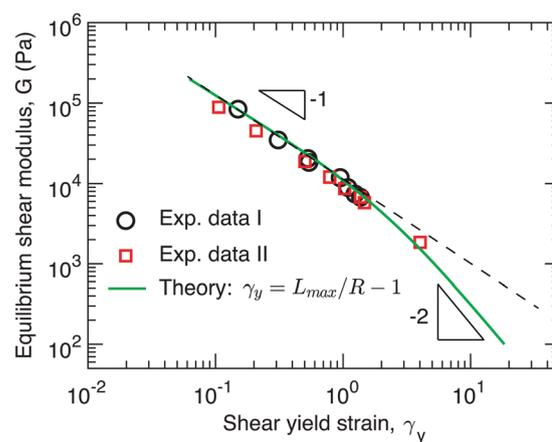
**Fig. 3** Dependence of stiffness on yield strain. The symbols are experimental data points extracted from Fig. 2a (circles) and Fig. 2b (squares). Solid line: theoretical prediction for the dependence of network stiffness  $G$  on the shear yield strain  $\gamma_y$  calculated based on  $\gamma_y = L_{\text{max}}/R - 1$  (eqn (1)), where both  $L_{\text{max}}$  and  $R$  are determined by the  $G$  (eqn (2), (3), (9), and (11)).
