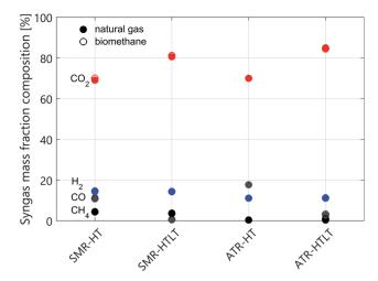
Fig. 1 Syngas composition of the four different hydrogen production pathways analysed. In red we show the CO<sub>2</sub> mass fraction, in blue the one of H<sub>2</sub>, in grey the one of CO and in black the one of methane. The full-dots represent the values obtained by reforming natural gas, while the empty circles represent the case with biomethane reforming.
