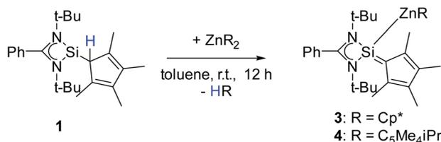
Scheme 4 Synthesis of  $\{[\text{PhC}(\text{NtBu})_2](\text{C}_5\text{Me}_4)\text{Si}\{\text{Zn}(\text{C}_5\text{Me}_5)\}\}$  (**3**) and  $\{[\text{PhC}(\text{NtBu})_2](\text{C}_5\text{Me}_4)\text{Si}\{\text{Zn}(\text{C}_5\text{Me}_4\text{iPr})\}\}$  (**4**).
