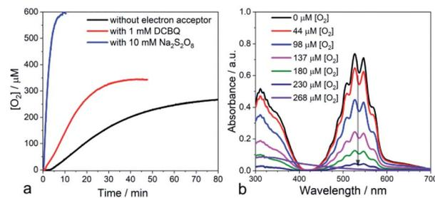
Fig. 4 (a) Time courses of oxygen evolution from water measured by a platinum Clark electrode in the absence of an electron acceptor (black) and in the presence of DCBQ (red) and S<sub>2</sub>O<sub>8</sub><sup>2-</sup> as electron acceptors (blue). (b) Titration of H<sub>2</sub>O<sub>2</sub> with KMnO<sub>4</sub> at different concentrations of photoproduct O<sub>2</sub> in the absence of an electron acceptor.
