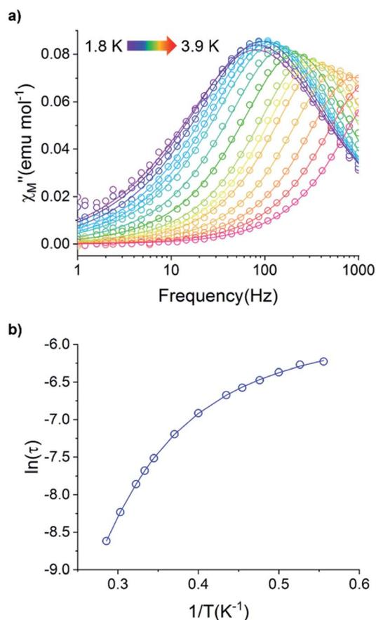
Fig. 12 (a) Temperature dependence of the out-of-phase component of the molar ac magnetic susceptibility ( $\chi_M''$ ) of **5**. ( $H = 0.2$  T,  $T = 1.8-3.9$  K). (b) Arrhenius plot of the magnetic relaxation time of **5**.
