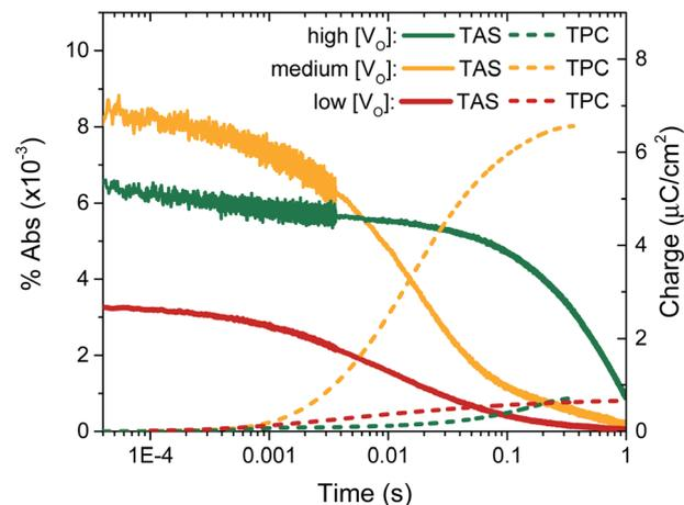
Fig. 4 Electron decays (solid lines, 800 nm) under bias (1.23  $\text{V}_{\text{RHE}}$ ) from transient diffuse reflectance spectroscopy measurements in 0.1 M  $\text{H}_2\text{SO}_4$ , exciting at 355 nm with 0.25  $\text{mJ cm}^{-2}$ . The transient photocurrent was measured simultaneously and then integrated to give the transient charge collected (dashed lines). The high performing sample with 'medium' doping (yellow) is compared to samples of 'high' (green) and 'low' doping (red).
