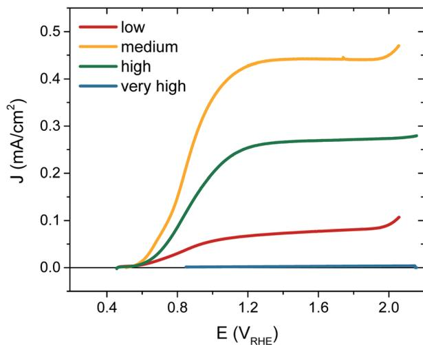
Fig. 3 Photocurrent responses for each  $\text{WO}_3$  sample under simulated 1 sun illumination from the front side in 0.1 M  $\text{H}_2\text{SO}_4$ , scan rate 10  $\text{mV s}^{-1}$ . Data given for 'very high'  $[\text{V}_\text{O}]$  (blue), 'high'  $[\text{V}_\text{O}]$  (green), 'medium'  $[\text{V}_\text{O}]$  (yellow) and 'low'  $[\text{V}_\text{O}]$  (red).
