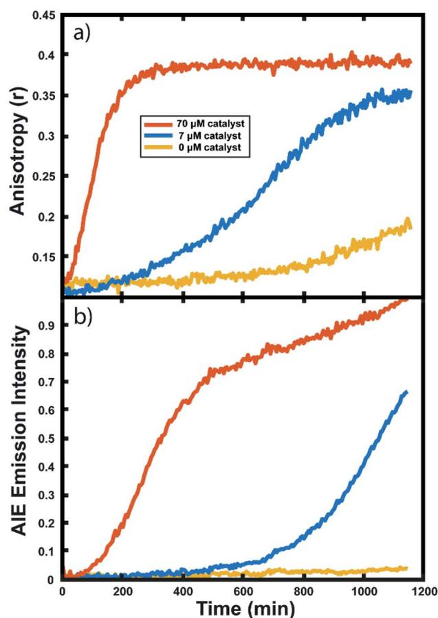
Fig. 6 Monitoring norbornene/norbornadiene droplets at different catalyst concentrations: (a) anisotropy response curves and (b) AIE response curves in droplets containing 70  $\mu\text{M}$  (red), 7  $\mu\text{M}$  (blue), and 0  $\mu\text{M}$  (yellow) Grubbs Gen II catalyst.
