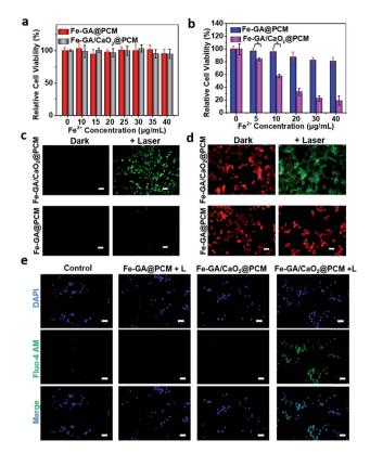
Fig. 2 (a) Dark cytotoxicity of Fe–GA/CaO<sub>2</sub>@PCM NPs and Fe–GA@PCM NPs on HeLa cells. (b) Cytotoxicity of HeLa cells of Fe–GA/CaO<sub>2</sub>@PCM NPs and Fe–GA@PCM NPs at different concentrations under laser irradiation. \*P < 0.001. (c) Intracellular hydroxyl radical detection with the DCFH-DA probe. (d) Mitochondrial membrane potential staining with the JC-1 probe. (e) Intracellular Ca<sup>2+</sup> detection with the Fluo-4 AM probe. Scale bars: 100  $\mu$ m.
