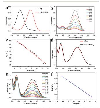
Fig. 7 UV-Vis spectra of 4-NP before and after adding NaBH<sub>4</sub> (a), UV-Vis spectra for the catalytic reduction of 4-NP (b), plots of  $\ln(C_t/C_0)$  versus t for the catalytic reduction of 4-NP (c), UV-Vis spectra of 2-NA before and after adding NaBH<sub>4</sub> (d), UV-Vis spectra for the catalytic reduction of 2-NA (e), plots of  $\ln(C_t/C_0)$  versus t for the catalytic reduction of 2-NA (f).
