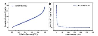
Fig. 5 Nitrogen adsorption—desorption isotherms of CS/GA/RGO/Pd hydrogel (a), and pore size distributions of CS/GA/RGO/Pd hydrogel (b).
