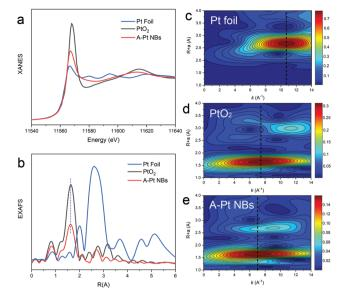
Fig. 3 X-ray absorption spectrometric studies of the A-Pt NBs. (a) XANES spectra at the Pt L<sub>3</sub>-edge of the A-Pt NBs, PtO<sub>2</sub>, and Pt foil. (b) Fourier transform (FT) EXAFS spectrum of the A-Pt NBs compared with PtO<sub>2</sub> and Pt foil at the Pt L<sub>3</sub>-edge. (c-e) Wavelet transform (WT) EXAFS of the Pt foil (c), PtO<sub>2</sub> (d) and A-Pt NBs (e).
