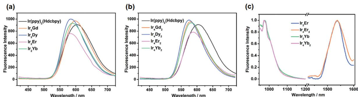
Fig. 7 (a) The emission spectra of Ir(ppy)<sub>2</sub>(Hdc bpy) and Ir<sub>2</sub>Ln in the solid-state ( $\lambda_{ex} = 375$  nm). (b) The emission spectra of Ir(ppy)<sub>2</sub>(Hdc bpy) and Ir<sub>4</sub>Ln<sub>2</sub> (Ln = Gd, Dy, Er, Yb) in the solid-state ( $\lambda_{ex} = 375$  nm). (c) The solid-state NIR emission spectra of the Ir–Yb (left) and Ir–Er (right) complexes ( $\lambda_{ex} = 500$  nm).
