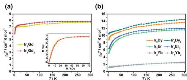
**Fig. 4** (a) Temperature dependence of  $\chi_{\text{M}}T$  per Gd on cooling in a field of 1 kOe for  $\text{Ir}_2\text{Gd}$  and  $\text{Ir}_4\text{Gd}_2$ . Inset:  $M$  vs.  $H$  plots of the two compounds at 2 K. (b) Temperature dependence of  $\chi_{\text{M}}T$  per Ln on cooling in a field of 1 kOe for  $\text{Ir}_2\text{Ln}$  and  $\text{Ir}_4\text{Ln}_2$  (Ln = Dy, Er, and Yb).
