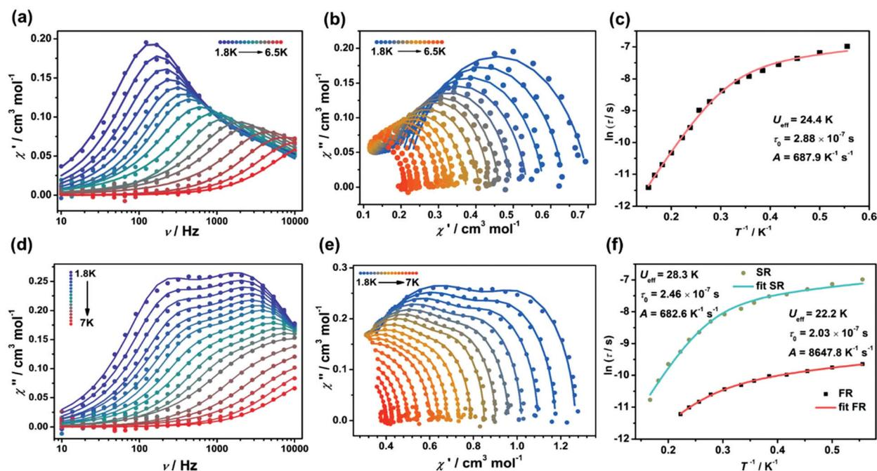
Fig. 6 Frequency dependence of out-of-phase ( $\chi''$ ) ac susceptibilities at different temperatures for  $\text{Ir}_2\text{Yb}$  (a) and  $\text{Ir}_4\text{Yb}_2$  (d) under an external dc field. The Cole–Cole plots of the ac susceptibilities for  $\text{Ir}_2\text{Yb}$  (b) and  $\text{Ir}_4\text{Yb}_2$  (e). Plots of  $\ln(\tau)$  vs.  $1/T$  for  $\text{Ir}_2\text{Yb}$  (c) and  $\text{Ir}_4\text{Yb}_2$  (f).
