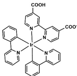
**Scheme 1** The molecular structure of the metalloligand Ir(ppy)<sub>2</sub>(Hdcppy).
