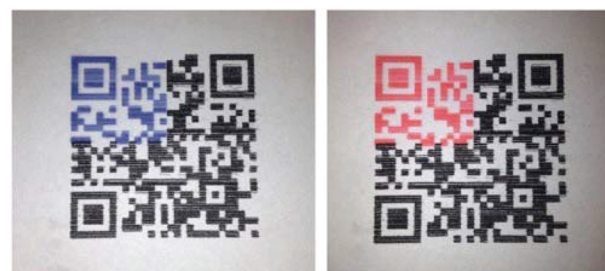
Fig. 17 QR code with partial area of TCDA/ZnO fabricated by inkjet printing methods to serve as a time temperature indicator. Reproduced from ref. 59 with permission from Elsevier, copyright [2014].
