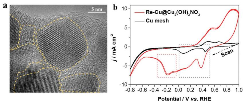
Fig. 5 (a) HRTEM image of the Re-Cu@Cu<sub>2</sub>(OH)<sub>3</sub>NO<sub>3</sub> nanodendrite and (b) cyclic voltammograms of the Re-Cu@Cu<sub>2</sub>(OH)<sub>3</sub>NO<sub>3</sub> and bare Cu mesh electrodes in 0.1 M KHCO<sub>3</sub> (saturated with Ar) for four segments respectively, without stirring, scan rate: 20 mV s<sup>-1</sup>.
