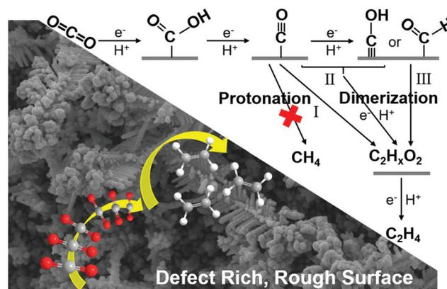
Fig. 6 Proposed pathway for the electroreduction of CO<sub>2</sub> to ethylene on the Re-Cu@Cu<sub>2</sub>(OH)<sub>3</sub>NO<sub>3</sub> electrode.
