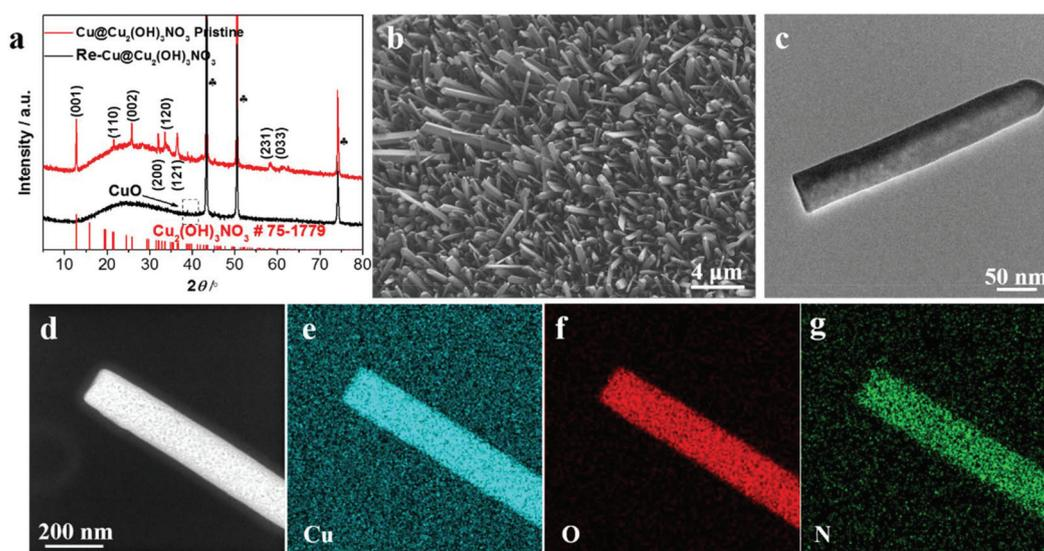
**Fig. 1** (a) XRD patterns of the  $Cu@Cu_2(OH)_3NO_3$  electrode before (red) and after (black) pre-reduction, (b) SEM and (c) TEM images of the pristine  $Cu@Cu_2(OH)_3NO_3$  electrode, (d) HAADF-STEM image and the corresponding elemental mapping images of (e) Cu, (f) O, and (g) N.
