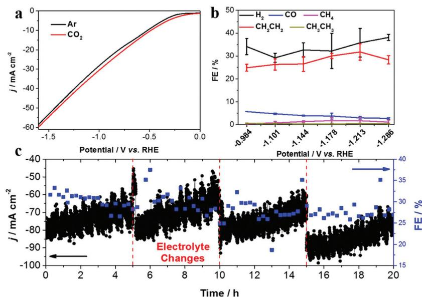
**Fig. 4** (a) LSV curves of the Re-Cu@Cu<sub>2</sub>(OH)<sub>3</sub>NO<sub>3</sub> electrode in Ar (black) and CO<sub>2</sub> (red) saturated 0.1 M KHCO<sub>3</sub> solution, without stirring, scan rate: 20 mV s<sup>-1</sup>, (b) the FE of the gaseous products as a function of applied potentials on the Re-Cu@Cu<sub>2</sub>(OH)<sub>3</sub>NO<sub>3</sub> electrode, and (c) long-term stability at -1.213 V (vs. RHE) of the Re-Cu@Cu<sub>2</sub>(OH)<sub>3</sub>NO<sub>3</sub> electrode.
