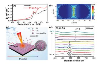
Fig. 2 (a) CO stripping voltammograms for Pt and Pt-on-Au core-satellite nanocatalysts in 0.1 M HClO<sub>4</sub> at a scan rate of 20 mV s<sup>-1</sup>. (b) 3D-FDTD simulation for a pair of Pt-on-Au nanocomposites. (c) A schematic diagram of the in situ electrochemical SERS study of CO electrooxidation. (d) The electrochemical SERS spectra for CO electrooxidation in 0.1 M HClO4 on Pt (2.1 nm)-on-Au core-satellite nanocatalysts.
