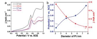
Fig. 3 (a) CO stripping voltammograms for Pt-on-Au core-satellite nanocatalysts with different Pt nanoparticle sizes in 0.1 M HClO<sub>4</sub> at a scan rate of 20 mV s<sup>-1</sup>. (b) The corresponding current density of the CO stripping peak and onset potentials of CO electrooxidation as a function of the Pt particle size.
