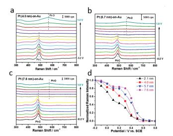
Fig. 4 (a)-(c) are the electrochemical SERS spectra for CO electrooxidation in 0.1 M HClO<sub>4</sub> on Pt-on-Au with a Pt particle size of 4.0 nm, 5.7 nm, and 7.6 nm, respectively. (d) Normalized Raman intensity of Pt-CO bands as a function of the potential.
