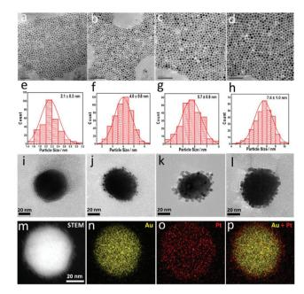
Fig. 1 (a)-(d) TEM images of Pt nanoparticles with different sizes. Their size distributions are shown in (e)-(h), respectively. (i)-(l) TEM images of the Pt-on-Au satellite nanostructure catalysts. 55 nm Au NPs (larger particles) are surrounded by Pt NPs (smaller ones) shown in (a)-(d) via electrostatic self-assembly. (m)-(p) High-angle annular dark field scanning transmission electron microscopy (HAADF-STEM) image and elemental maps of Pt (2.1 nm)-on-Au.
