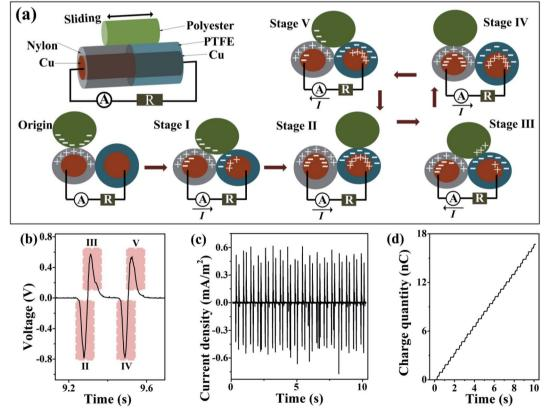
Fig. 2 (a) Working mechanism of the FTNG under a lateral sliding mode. (b) Enlarged output voltage of the FTNG a under frequency of 1.8 Hz with the displacement of 10 mm. (c) The current density of FTNG via dividing the output current in Fig. S1e† by the contact area. (d) The accumulative charge quantity via integrating the output current in Fig. S1e.†
