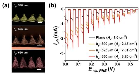
Fig. 4 (a) Optical images of the fabricated 3D photoelectrodes composed of 400 pyramids. The total light absorption area  $(A_a)$  of the 3D photoelectrodes is modulated by adjusting  $h_p$  to 390, 525, and 650  $\mu$ m (fixed  $L_b$ : 490  $\mu$ m). The scale bar is 250  $\mu$ m. (b) Chopped-light PEC performance of the p-n homojunction Cu<sub>2</sub>O electrodes with planar and 3D pyramid shapes with respect to the total light absorption area  $(A_a)$ .
