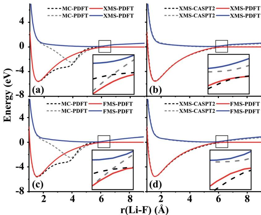
Fig. 1 Comparison of the potential energy curves of the two lowest  $A_1$  electronic states of LiF with (a) XMS-PDFT and MC-PDFT, (b) XMS-PDFT and XMS-CASPT2, (c) FMS-PDFT and MC-PDFT, and (d) FMS-PDFT and XMS-CASPT2. The area near the avoided crossing (indicated by a small box) for each curve is also shown magnified.
