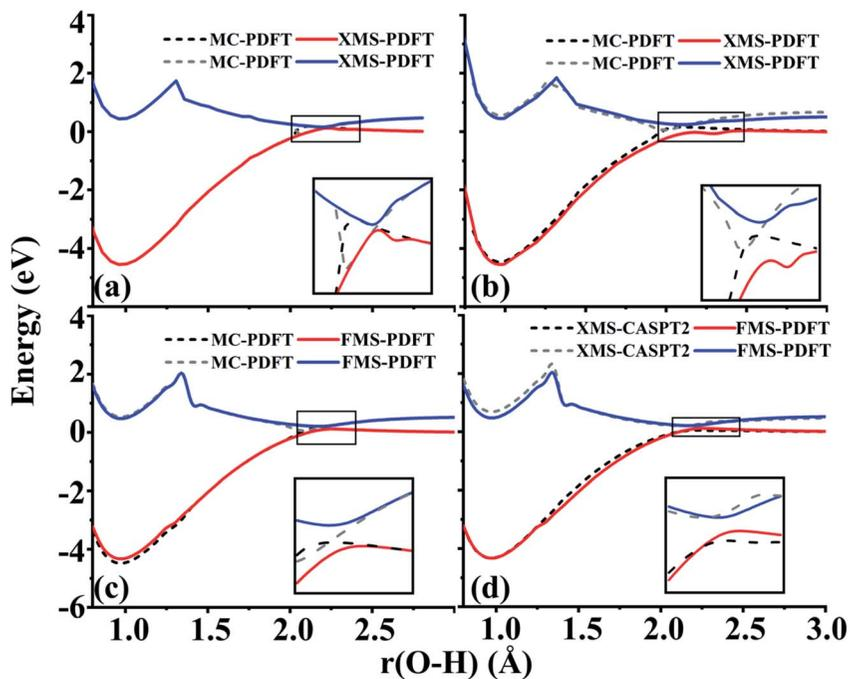
Fig. 5 (a) and (b) Potential energy curves of two states for O–H dissociation in phenol with H–O–C–C dihedral angles of  $1^\circ$  and  $10^\circ$ , calculated by MC-PDFT (dashed and dotted lines) and XMS-PDFT (solid lines). (c) and (d) Potential energy curves for two states with an H–O–C–C dihedral angle of  $10^\circ$  calculated by FMS-PDFT compared with those calculated by MC-PDFT and XMS-CASPT2.
