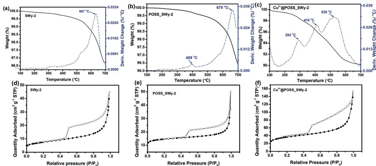
Fig. 4 Thermogravimetric analysis (TGA) and differential thermal analysis (DTA) data for (a) SWy-2, (b) POSS\_SWy-2 and (c)  $\text{Cu}^{2+}$ @POSS\_SWy-2.  $\text{N}_2$  adsorption-desorption isotherms of SWy-2 (d), POSS\_SWy-2 (e) and  $\text{Cu}^{2+}$ @POSS\_SWy-2 (f).
