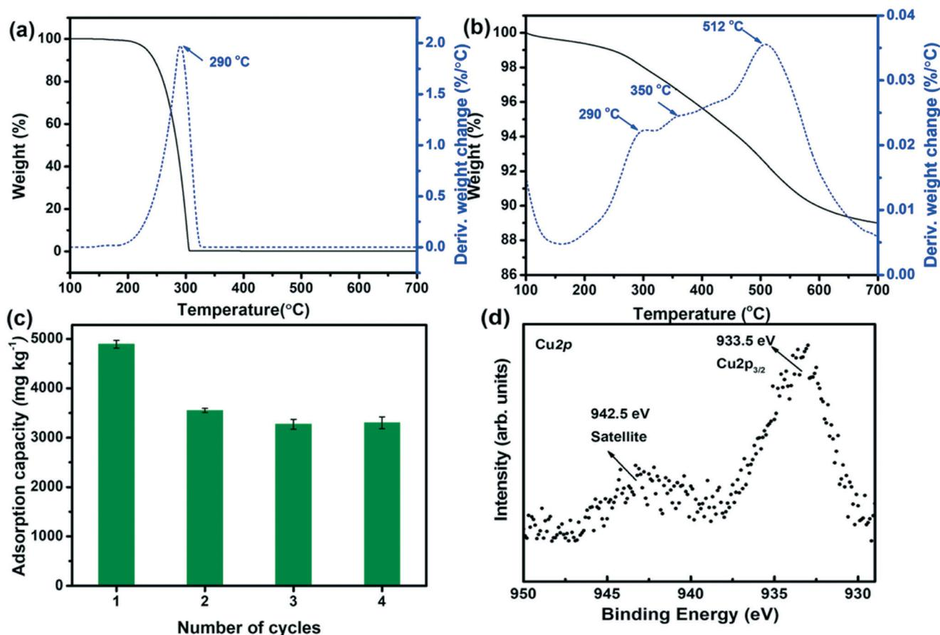
Fig. 6 Thermogravimetric analysis (TGA) and differential thermal analysis (DTA) data for (a) chloridazon and (b) Cu<sup>2+</sup>@POSS\_SWy-2 + chloridazon, and (c) adsorption capacity for chloridazon of Cu<sup>2+</sup>@POSS\_SWy-2 after an increasing number of thermal regeneration cycles. (d) X-ray photoelectron spectrum of the Cu<sub>2p<sub>3/2</sub></sub> core level region of thermally regenerated Cu<sup>2+</sup>@POSS\_SWy-2.
