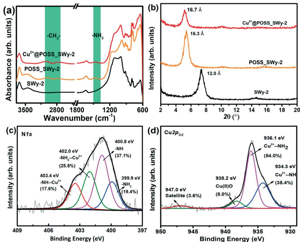
Fig. 1 (a) FTIR spectra and (b) XRD spectra of SWy-2, POSS\_SWy-2 and Cu<sup>2+</sup>@POSS\_SWy-2; X-ray photoelectron spectra of Cu<sup>2+</sup>@POSS\_SWy-2 (c) N1s and (d) Cu2p<sub>3/2</sub> core level regions.
