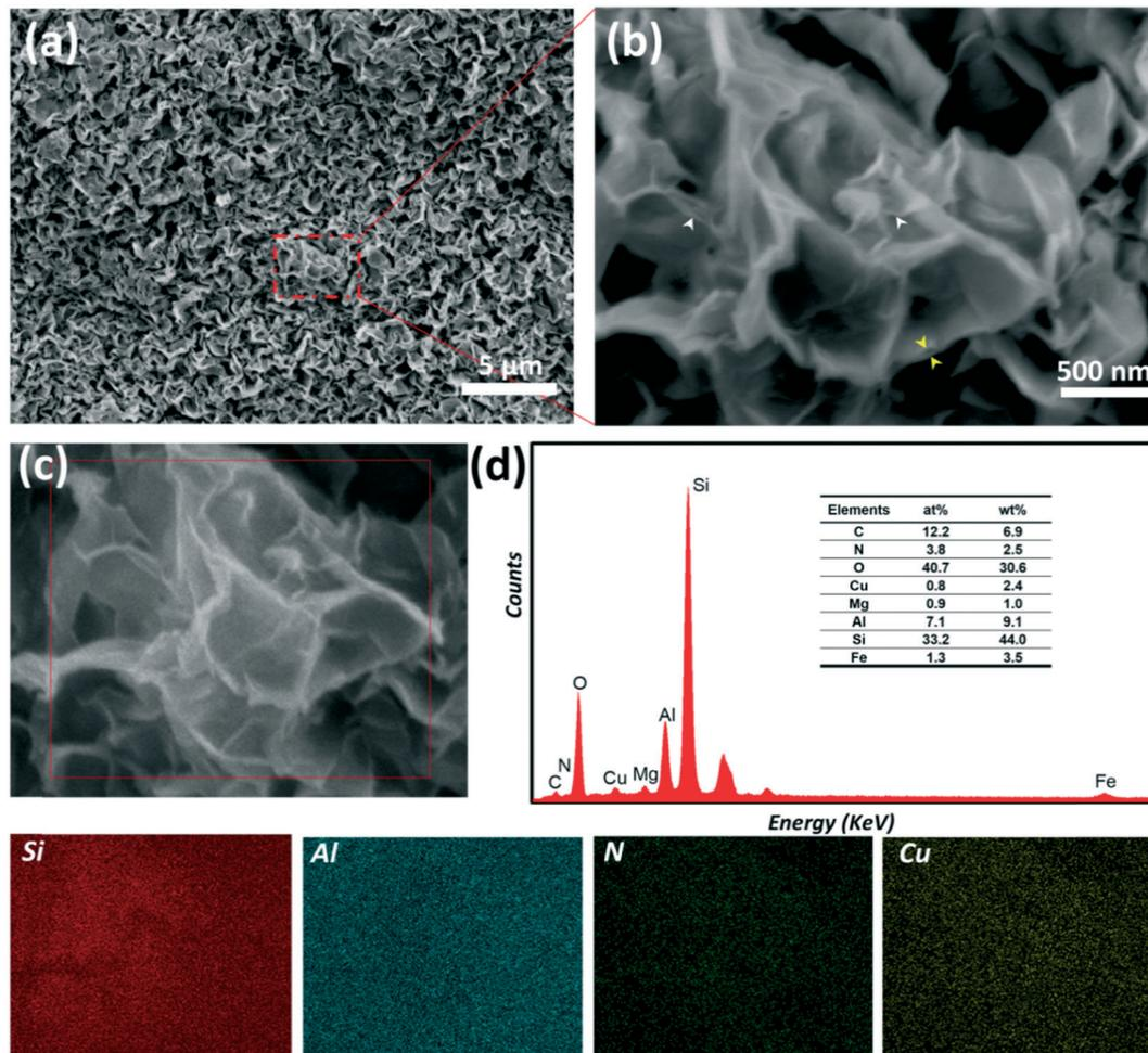
Fig. 3 (a) and (b) SEM images of  $\text{Cu}^{2+}$ @POSS\_SWy-2. (c) SEM image with the area selected for energy dispersive X-ray spectroscopy (EDS) spectra and EDS elemental mapping measurement marked in red. (d) SEM-EDS spectra of  $\text{Cu}^{2+}$ @POSS\_SWy-2. Inset: The elemental composition results. The bottom panels show the EDS elemental mapping results for Si, Al, N and Cu in  $\text{Cu}^{2+}$ @POSS\_SWy-2 based on the red square area in (c).
