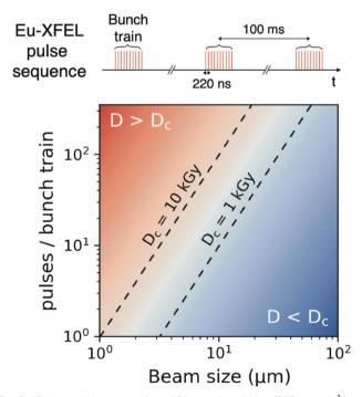
Fig. 5 Estimated X-ray dose for a BSA protein solution (250 mg ml $^{-1}$ ) as a function of beam size and number of pulses per bunch train. The upper panel shows the European XFEL pulse sequence, where the pulses have a minimum separation of 220 ns and the bunch trains are separated by 100 ms. The lower panel shows the dose estimate for a standard configuration at the MID instrument of Eu-XFEL, where a typical critical doses of protein solutions of 1 kGy to 10 kGy are denoted with dashed lines.
