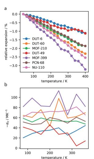
Fig. 2 Relative expansion of the investigated MOFs (a). Volumetric thermal expansion coefficient,  $\alpha_V$ , calculated over the temperature range, computed for intervals of 40 K (b).
