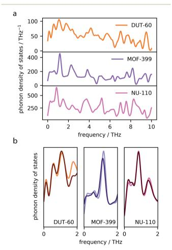
Fig. 4 Phonon density of states for DUT-60, MOF-399 and NU-110 computed by finite-displacement and harmonic approximation (a). A comparison of the lowest frequency modes at volumes corresponding to 40 and 300 K, where the density of states at 300 K is indicated by a darker color (b).
