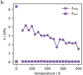
Fig. 6 Directional Young's modulus of MOF-399 computed for trajectories at 40 and 400 K (a). Maximum and minimum ( $\lambda_{max}$  and  $\lambda_{min}$ ) eigenvalues of the stiffness matrix for MOF-399 over the studied temperature range (b). The values at 0 K correspond to density functional theory simulations reported previously.<sup>14</sup>
