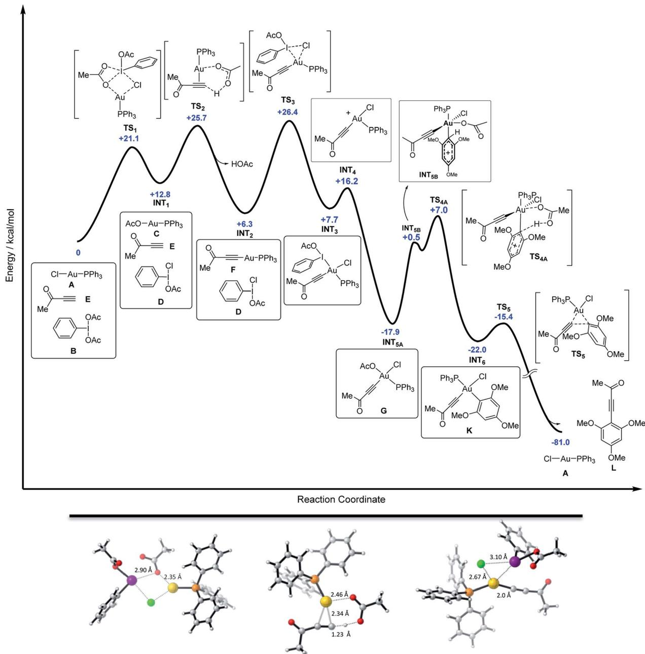
Fig. 5 Top: complete energy profile for the reaction between  $\text{Ph}_3\text{PAuCl}$ , alkyne (methyl alkynyl ketone),  $\text{PhI}(\text{OAc})_2$  and arene (1,3,5-trimethoxybenzene). Gibbs free energy values in blue calculated with the M06 functional. Bottom: structures of transition states  $\text{TS}_1$ ,  $\text{TS}_2$  and  $\text{TS}_3$  (left to right) highlighting the relevant distances.
