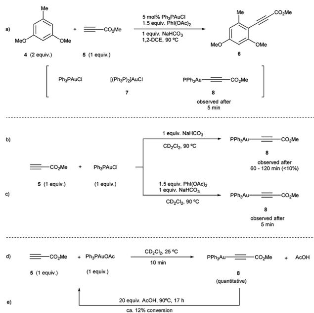
Fig. 2 (a) Standard catalytic reaction. (b and c) Experiments towards the formation of Au(I)-acetylide 8 from  $\text{Ph}_3\text{PAuCl}$  and alkyne 5 in the absence or presence of  $\text{PhI}(\text{OAc})_2$ , respectively. (d and e) Reactivity of  $\text{Ph}_3\text{PAuOAc}$  towards methyl propiolate (5).
