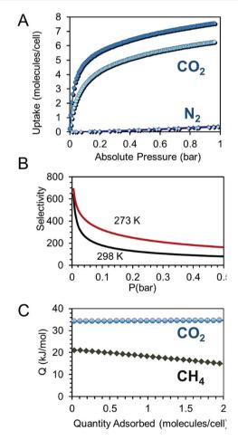
Fig. 2 (A) CO<sub>2</sub> and N<sub>2</sub> isotherms of CPOS-5 collected at 273 K (blue circles and diamonds, respectively) and 298 K (light-blue circles and diamonds, respectively). (B) CO<sub>2</sub>/N<sub>2</sub> selectivity values of CPOS-5 *versus* pressure calculated starting from a 15/85 mixture and applying IAST calculation. (C) Isosteric heats of adsorption ( $Q_{\rm st}$ ) *versus* CO<sub>2</sub> and CH<sub>4</sub> loading.
