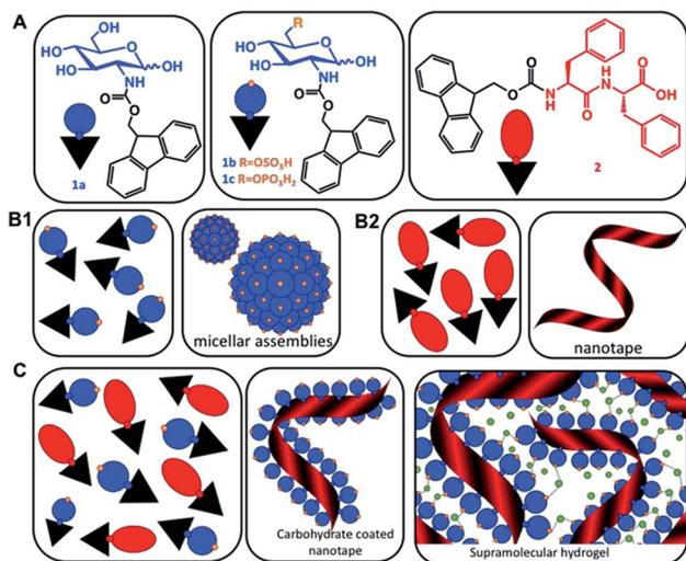
**Scheme 1** (A) Chemical structures of the carbohydrate amphiphiles (**1**) and the peptide analogue Fmoc-FF (**2**). (B) Schematic representation of the assembly of the individual components (**1**) and (**2**) in water resulting in the formation of micelles and nanotapes, respectively. (C) Co-assembly of (**1**) and (**2**) to form carbohydrate functionalized peptide nanotapes and supramolecular hydrogels. Green dots represent divalent cations.
