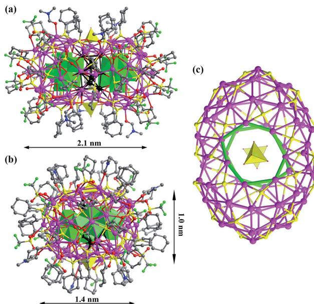
Fig. 1 (a) and (b) The X-ray crystal structure of Ag<sub>10</sub>@(Mo<sub>7</sub>O<sub>26</sub>)<sub>2</sub>@Ag<sub>70</sub> nanoclusters viewed along two orthogonal directions. The inner silver atoms of the Ag<sub>10</sub> kernel are highlighted in black. Mo<sub>7</sub>O<sub>26</sub><sup>10−</sup> and MoO<sub>4</sub><sup>2−</sup> are represented by green and yellow polyhedra, respectively. (c) The Ag<sub>70</sub>S<sub>36</sub> shell with silver heptagons highlighted in green.
