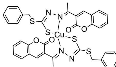
Fig. 1 Copper complex synthesised with *S*-benzylthiocarbamate and 3-acetylcoumarin [Cu(SBCM)<sub>2</sub>].
