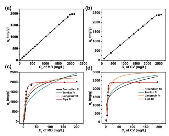
Fig. 10 The variation of the amount of dye adsorbed at equilibrium by Dex-MA/PAA,  $q_e$ , with initial dye concentrations,  $C_0$ , for (a) MB and (b) CV. The fitting curves for the Freundlich, Temkin, Langmuir and Sips isotherms for (c) MB and (d) CV. Dex-MA/PAA dose: 1 g L<sup>-1</sup>, pH<sub>initial</sub> 8.0.
