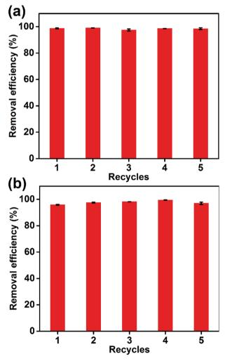
Fig. 11 Removal efficiencies for (a) MB and (b) CV were >95% after five Dex-MA/PAA hydrogel adsorption/desorption cycles. Dex-MA/PAA hydrogel dose:  $1 \text{ q L}^{-1}$ , dye concentration:  $50 \text{ mg L}^{-1}$ ,  $pH_{\text{initial}}$  8.0.
