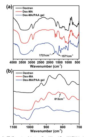
Fig. 2 FT-IR spectra of dextran, Dex-MA and Dex-MA/PAA hydrogel.
