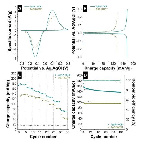
Fig. 3 Electrochemical characterization using a half-cell setup and 1 M NaCl for AgNP-10CB and AgCl-20CNT electrodes. (A) Cyclic voltammetry at 1 mV s<sup>-1</sup>, (B) galvanostatic charge/discharge at 0.1 A  $g^{-1}$ , (C) galvanostatic rate handling at 0.1–10 A  $g^{-1}$ , and (D) galvanostatic charge/discharge cycling stability at 0.25 A  $g^{-1}$ .
