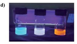
Fig. 1 (a) PL spectra of Si QDs after addition of different volumes of Au NCs; (b) corresponding chromaticity plot for color co-ordinates; (c) digital images of Si QDs, WLEM and Au NCs in day light; and (d) digital images of Si QDs, WLEM and Au NCs under UV light ( $\lambda_{ex} = 365 \text{ nm}$ ).
