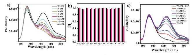
Fig. 5 (a) PL spectra of WLEM upon addition of different concentration of  $Hg^{2+}$  ions; and (b) change in PL intensity of Si QDs (black) and Au NCs (pink) in the WLEM upon addition of different ions; and (c) PL spectra of WLEM having  $Hg^{2+}$  ions with different concentration of Cys.
