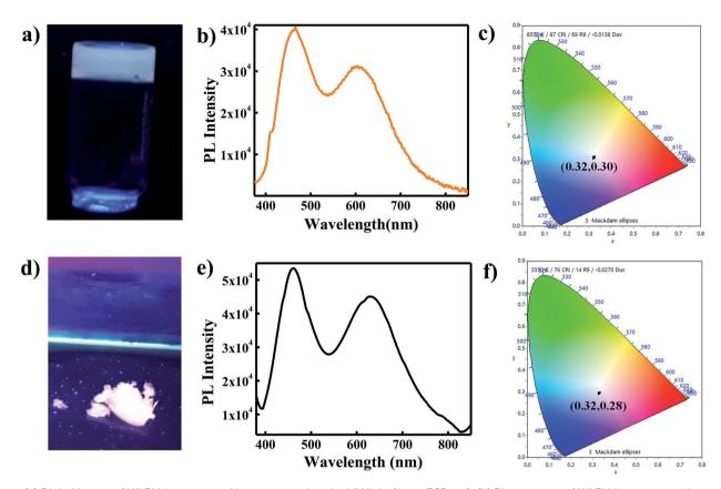
Fig. 4 (a) Digital image of WLEM incorporated in agarose gel under UV light ( $\lambda_{ex} = 365$  nm); (b) PL spectrum of WLEM incorporated in agarose gel; (c) corresponding chromaticity plot for color co-ordinate; (d) digital image of WLEM incorporated in powder form under UV light ( $\lambda_{ex} = 365$  nm); (e) PL spectrum of WLEM incorporated in powder form; and (f) corresponding chromaticity plot for color co-ordinate.
