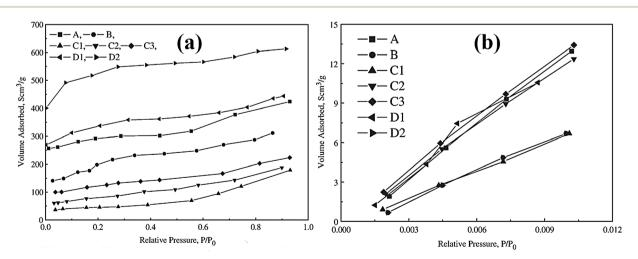
Fig. 1 N<sub>2</sub> and CO<sub>2</sub> adsorption isotherms of the activated carbon produced from different starting materials.<sup>26</sup> This figure has been adapted from ref. 26 with permission from Elsevier.
