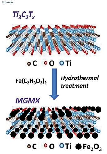
Fig. 8 Schematic structure of the composite formed by MXenes and Fe<sub>2</sub>O<sub>3</sub>.<sup>22</sup> This figure has been adapted from ref. 22 with permission from Elsevier.
