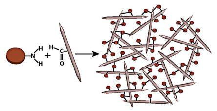
Fig. 7 Schematic of the preparation of the chemically crosslinked CNC/GQD hydrogel.<sup>95</sup> This figure has been adapted from ref. 95 with permission from ACS Nano.
