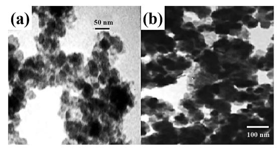
Fig. 6 TEM image of (a) MIONPs and (b) M-MIONPs.<sup>56</sup> This figure has been adapted from ref. 66 with permission from Elsevier.
