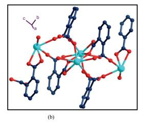
Fig. 1 (a) The coordination environments of Pr(III) ions in the asymmetric unit in 1. (b) Diamond representation of tetranuclear clusters connected by carboxylic groups.
