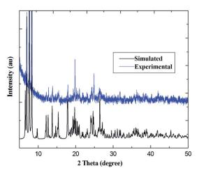
Fig. 3 Comparison of simulated and experimental PXRD patterns for  $Pr(\mbox{\tiny III})$  compound 1.
