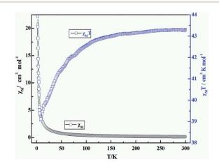
Fig. 11 Temperature dependence of  $\chi_M T$  ( $\square$ ) and  $\chi_M$  ( $\bigcirc$ ) *versus T* for coordination polymer **3** under the magnetic field of 1000 Oe.
