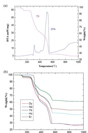
Fig. 4 (a) The TG-DTA diagrams of coordination polymer 1. (b) TG curves of coordination polymers 2–6.
