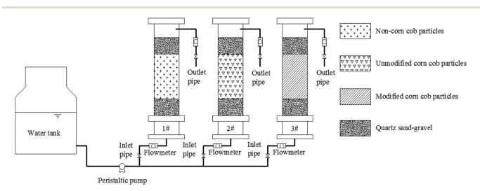
Fig. 1 System diagram of dynamic testing device.
