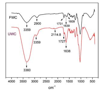
Fig. 12 FTIR spectra of fresh wood (FWC) and used wood (UWC).
