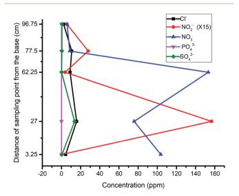
Third run of nitrite-spiked well water in the modified column.
