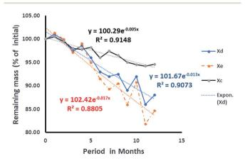
**Fig. 13** Rate of degradation of date seed: Xd is the entire date, Xc is the cover wall of the seed, and Xe is the deduced degradation pattern of the endosperm.
