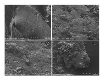
Fig. 9 FESEM images of (a) fresh date seed (10  $\mu$ m), (b) used date seed (10  $\mu$ m), (c) used date seed (5  $\mu$ m), (d) used date seed (20  $\mu$ m).
