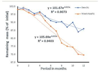
Fig. 14 Comparative rates of degradation of date seed and wood chips in the same column.
