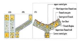
Fig. 1 Order of the sequence multi-barrier reactive media in the funnel and gate. (Q) the column packing structure, (R) the alignment of the column packing structure with respect to the geometry of the funnel and gate, and (S) the funnel and gate. A, B, C and D are compartments as described.
