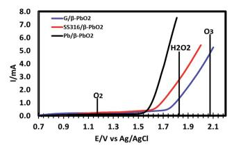
Fig. 3 LSV grame of  $\beta$ -PbO<sub>2</sub> electrodes in Na<sub>2</sub>SO<sub>4</sub> (0.25 M) at pH = 6.0. Scan rate = 100 mV s<sup>-1</sup>.
