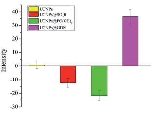
Fig. 2 Zeta potential of UCNPs, UCNPs@SO $_3$ H, UCNPs@PO(OH) $_2$  and UCNPs@GDN.
