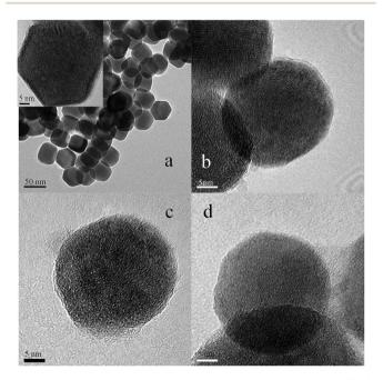
Fig. 1 TEM images of UCNPs (a), UCNPs@SO<sub>3</sub>H (b), UCNPs@PO(OH)<sub>2</sub> (c) and UCNPs@GDN (d).
