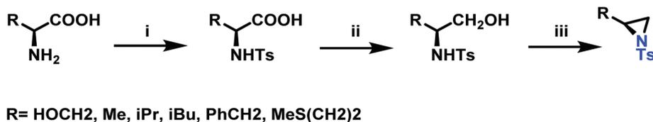
**Scheme 12** i: Preparation of *N*-tosyl-2-aminoacids via *N*-tosylation with TsCl; ii: preparation of *N*-tosyl-2-aminoalcohols reduction of the carbonyl group; iii: preparation of 2-substituted *N*-tosylaziridines.
