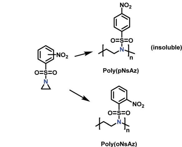
**Scheme 17** Azaanionic polymerization of nitrophenylsulfonyl-activated aziridines.<sup>141</sup>
