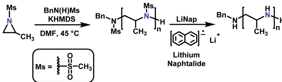
**Scheme 15** Anionic ring-opening polymerization of sulfonyl aziridines and subsequent desulfonylation (with 2-methyl-mesyloxyaziridine as an example).
