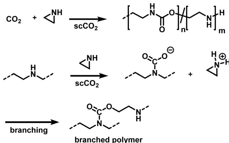
**Scheme 25** Copolymerization of aziridines and CO<sub>2</sub> to branched poly(urethane-*co*-amine)s.<sup>173,174</sup>
