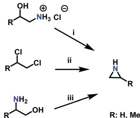
**Scheme 3** Synthesis of aziridines with and without a ring substituent (R) by i: the  $\beta$ -chloroethylamine process, ii: the Dow Process, iii: the Wenker synthesis.
