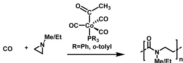
Scheme 27 Alternating copolymerization of alkylated aziridines and carbon monoxide towards well-defined poly- $\beta$ -peptides.<sup>177</sup>
