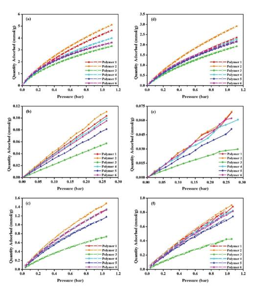
Fig. 5 Adsorption isotherms of  $CO_2$  (a),  $N_2$  (b),  $CH_4$  (c) gases at 273.15 K, and  $CO_2$  (d),  $N_2$  (e),  $CH_4$  (f) gases at 298.15 K for polymer 1 to polymer 6. Filled symbols represent adsorption and open symbols represent desorption.
