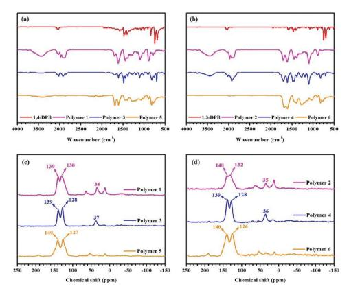
Fig. 1 FT-IR spectrum of (a) 1,4-DPB and 1,4-DPB-based polymer materials, and (b) 1,3-DPB and 1,3-DPB-based polymer materials; solid state cross-polarization (CP) <sup>13</sup>C MAS natural abundance NMR spectrum of (c) 1,4-DPB-based polymer materials, and (d) 1,3-DPB-based polymer materials.
