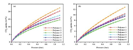
Fig. 4 (a) Volumetric CO<sub>2</sub> adsorption isotherms and desorption isotherms up to 1.13 bar at 273.15 K, and (b) volumetric CO<sub>2</sub> adsorption isotherms and desorption isotherms up to 1.13 bar at 298.15 K.
