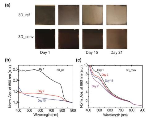
Fig. 5 Characterization of the moisture stability of the reference and converted 3D FAPbl<sub>3</sub> perovskite films under ambient conditions. (a) Photographs showing the evolution of the color of the reference (top) and converted (bottom) perovskite films over a 21 day period. (b and c) UV-vis absorbance spectra of the reference (b) and the converted (c) films normalized at 890 nm.
