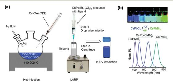
Fig. 3 Synthesis of colloidal PNCs and bandgap tuning via anion-exchange. Schematic diagrams of (a) the hot-injection method (left panel) and the LARP technique (right panel). (b) Photographs of colloidal CsPb(Br<sub>1-x</sub>Cl<sub>x</sub>)<sub>3</sub> PNC solutions under UV irradiation and their PL spectra, wherein emission shifts towards the deep blue region with higher chloride/bromide ratios. Reproduced with permission. Copyright © 2015 American Chemical Society.
