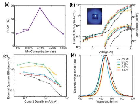
Fig. 5 Blue PeLEDs based on Mn-doped PNCs with various doping concentrations. (a) PLQEs of Mn-doped PNCs. (b) J-V-L characteristics; the inset image is a photograph of a blue LED under operation. (c) EQE-current density plots. (d) EL spectra. Reproduced with permission. <sup>57</sup> Copyright © 2018 Elsevier Inc.
