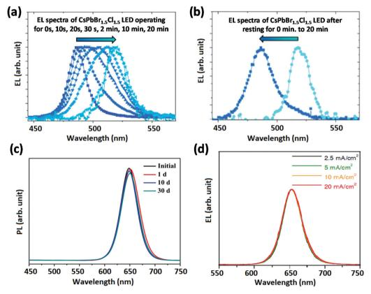
Fig. 6 Colour stability of blue PeLEDs. EL spectra recorded (a) after different time intervals and (b) after resting for 0/20 min. Reproduced with permission. Topyright © 2016, John Wiley and Sons. (c) PL spectra of  $CsPb(I_{1-x}Br_x)_3$  PNCs with a metal stearate solid matrix. Reproduced with permission. Copyright © 2018, American Chemical Society. (d) EL spectra under various current densities. Reproduced with permission. Pringer Nature.
