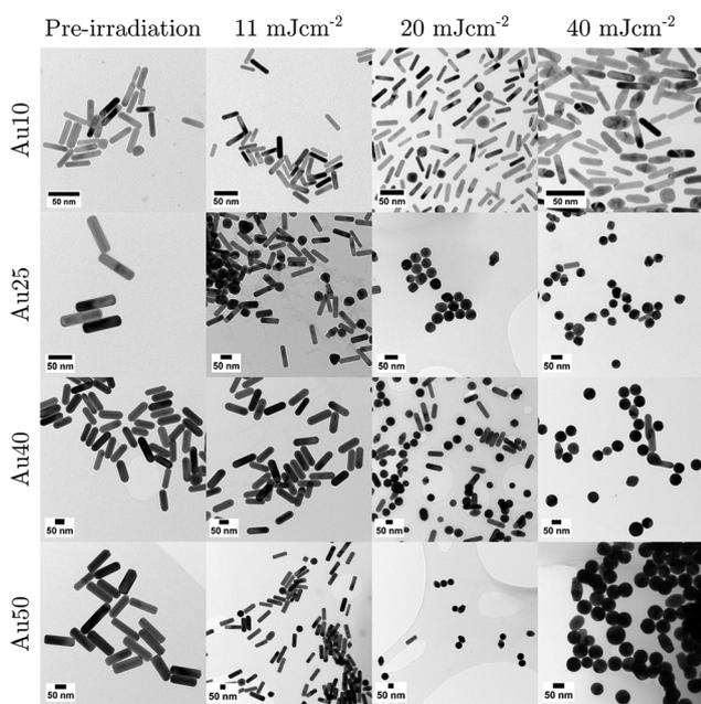
Fig. 4 TEM images taken for each sized AuNR at specific points in the study: before laser irradiation, and after 20 pulses at  $11$  mJ cm<sup>-2</sup>,  $20$  mJ cm<sup>-2</sup>, and  $40$  mJ cm<sup>-2</sup>. Scale bars = 50 nm.
