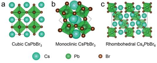
Fig. 1 Simulated crystal structure of (a) cubic  $CsPbBr_3$ , (b) monoclinic  $CsPbBr_3$  and (c) rhombohedral  $Cs_4PbBr_6$ .
