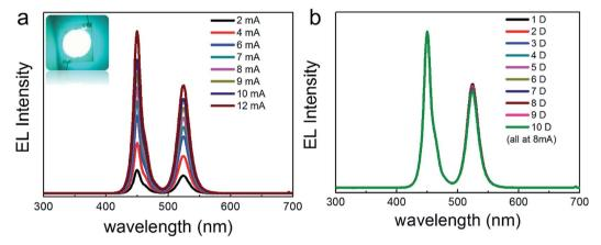
Fig. 9 (a) EL spectra of the CsPbBr $_3$ @Cs $_4$ PbBr $_6$  NC powder-based backlit LED under different currents; inset is the photograph of the backlit LED. (b) EL spectra of the CsPbBr $_3$ @Cs $_4$ PbBr $_6$ -based backlit LED lighted for 10 days under ambient conditions.
