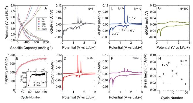
Fig. 4 Performance of composites of  $MoO_2$  flakes/SWCNTs (20 wt%) as lithium ion battery anodes. (A) Galvanostatic charge—discharge curves for different number of cycles. (B) Cycling (charging) capacity *versus* cycle number at 0.1 A g<sup>-1</sup> with coulombic efficiency shown in the inset. (C–G) Differential curves associated with voltage profiles for different cycle numbers. (H) Absolute heights for the peaks at 1.7 V (insertion) and 0.33 V (conversion).
