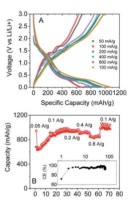
Fig. 5 (A) Galvanostatic charge-discharge curves measured at different current rates. (B) Capacity as a function of current rate with coulombic efficiency shown in the inset (discharge – open circles, charge – filled circles).
