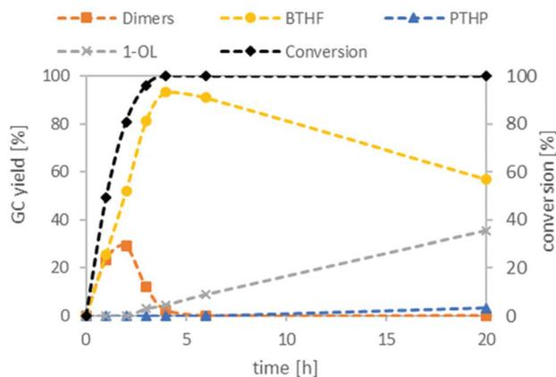
**Fig. 3** Reaction profile for the deoxygenation of THFA. THFA (7.5 mmol), Ru/C (0.038 mmol Ru), Amberlyst 36 (0.5 mmol H<sup>+</sup>), H<sub>2</sub> (80 bar), 150 °C, cyclohexane (15 mL).
