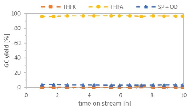
Fig. 7 Continuous Flow Hydrogenation of a FFA (0.25 mol L<sup>-1</sup>) solution in cyclohexane. Conditions: Catalyst bed: 1 g Ru/C, 50 °C, substrate flowrate: 1 mL min<sup>-1</sup>, hydrogen flowrate: 37 mL<sub>N</sub> min<sup>-1</sup>, pressure: 80 bar, WHSV = 2 h<sup>-1</sup>.
