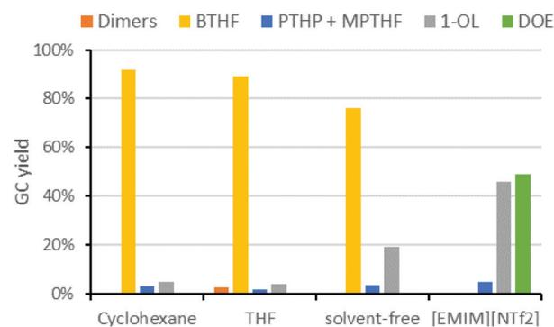
**Fig. 5** Influence of the solvent on the deoxygenation of THFA. Conditions: THFA (0.75 mmol), Ru/C (3.75 μmol Ru), Amberlyst-36 (9.3 mg, 0.05 mmol H<sup>+</sup>), H<sub>2</sub> (80 bar), 150 °C, 6 h, solvent (1.5 mL). [Emim][NTf<sub>2</sub>] = 1-ethyl-3-methylimidazolium bis(trifluoromethylsulfonyl)imide.
