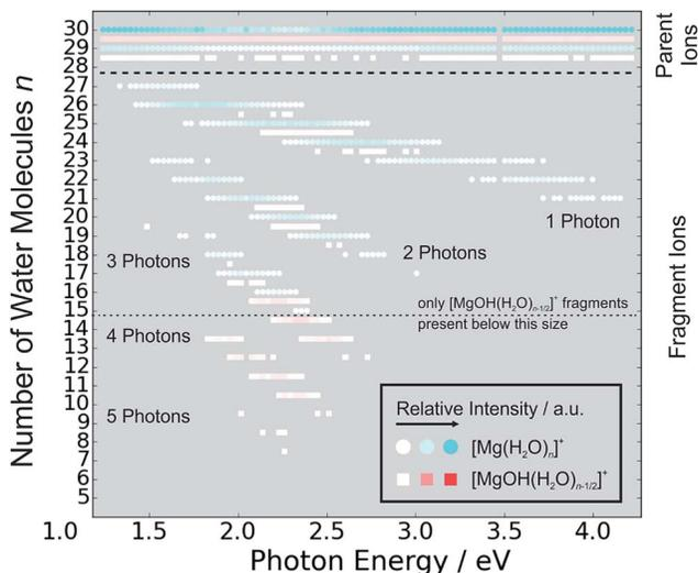
Fig. 5 Fragmentation pattern from a typical photodissociation experiment for  $[\text{Mg}(\text{H}_2\text{O})_{29,30}]^+$ . The two different species of hydrated magnesium ions are represented by blue dots for  $[\text{Mg}(\text{H}_2\text{O})_n]^+$  ions and red squares for  $[\text{MgOH}(\text{H}_2\text{O})_{n-1/2}]^+$  ions. Color intensity represents measured ion intensity.
