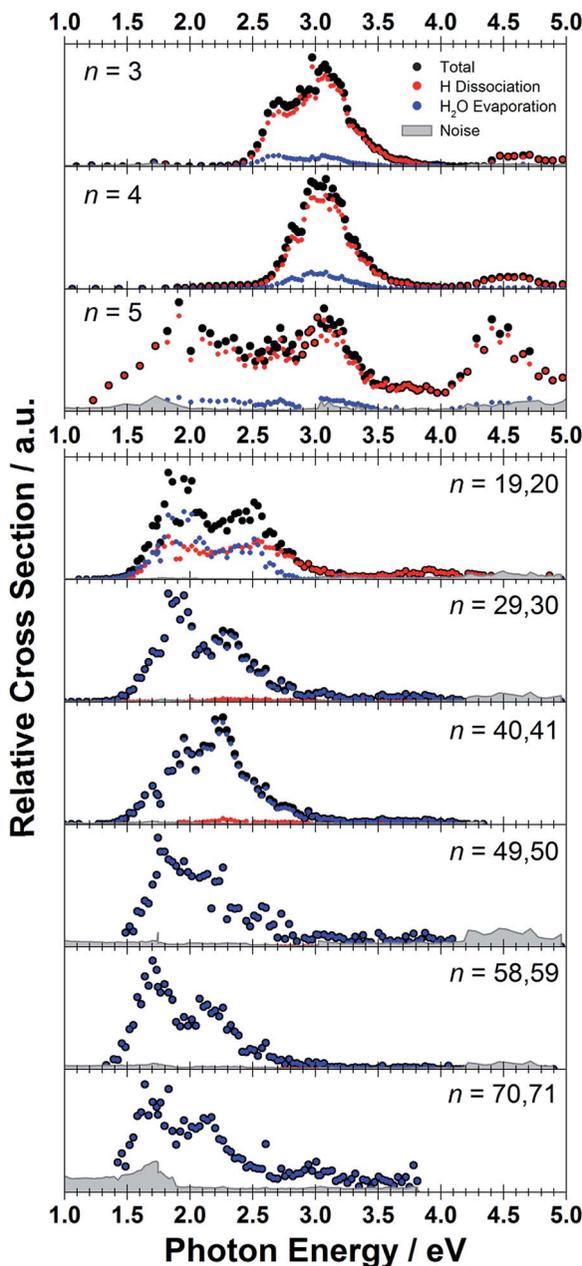
Fig. 1 Experimentally measured relative photodissociation cross sections of  $[\text{Mg}(\text{H}_2\text{O})_n]^+$  ions for  $3 \leq n \leq 5$  (adapted from ref. 42) and  $n \sim 20, 30, 40, 50, 60$  and  $70$ , with partial cross sections for fragmentation *via* only the loss of water molecules (blue) and the additional loss of atomic hydrogen (red).
