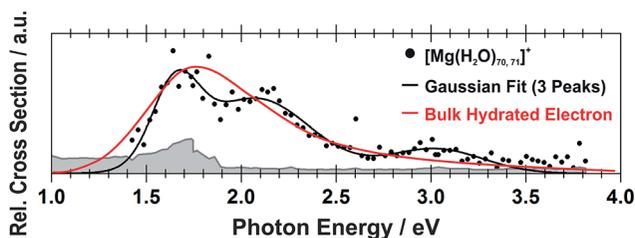
Fig. 4 Comparison between the photodissociation spectrum of  $[\text{Mg}(\text{H}_2\text{O})_{70,71}]^+$  and the spectrum of a bulk hydrated electron.<sup>73</sup>
